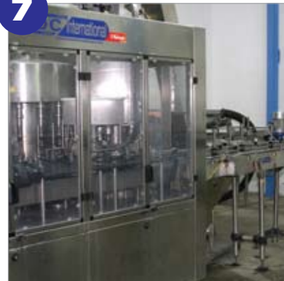
The washed bottles are filled with spring water in a sterile environment.
