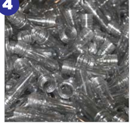
Preformed bottle blanks are fed into a hopper.
