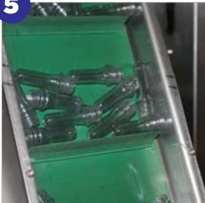
Bottle blanks travel to the blower which extrudes them into an 8-oz. or 16-oz. bottle.
