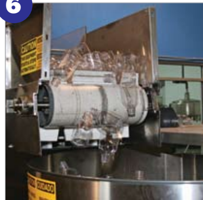
Formed bottles exit the blower and are thoroughly washed.
