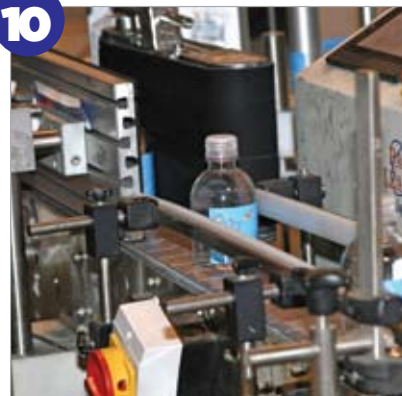
Bottles travel through the label applicator and are placed into cases.
